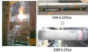
Fig. 2 Ingot making of VIM and ESR
