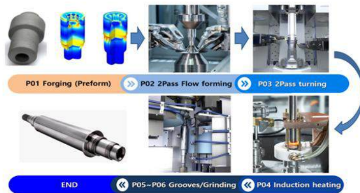
< Hollow shaft manufacturing process using flow forming>
